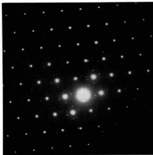
Fig. 3. Diffraction pattern of another specimen with (\bar{1}10) orientation at 20^\circ\text{C} . Here the two patterns of Fig. 2(b) and (c) are superposed.
